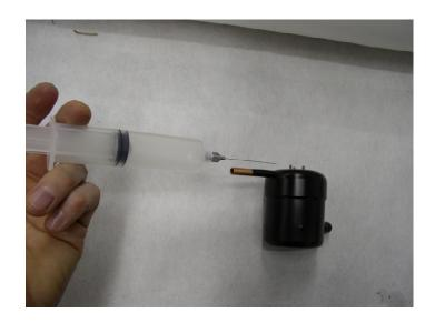
"Note" Syringe must have large enough ID to allow oil flow and a small enough OD to allow air to purge from canister.
